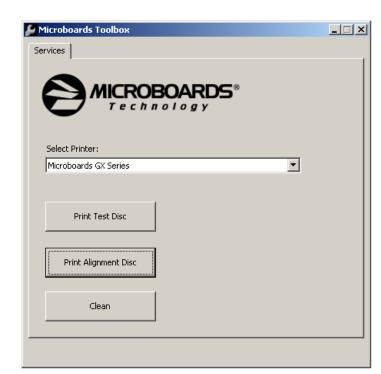
Place an alignment disc (provided) in the input hopper and click the **Print Alignment Disc** button. **Remember, the alignment CD should always be printed in Photo Best mode for the highest accuracy.**
